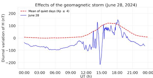
Figure 5. Effects of the geomagnetic storm on the diurnal variation of the horizontal component of Earth's magnetic field at the Jicamarca station on June 28, 2024.
