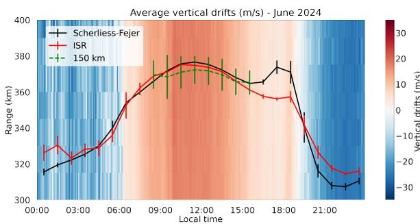
Figure 8. ISR monthly average vertical drifts for the June geomagnetic quiet days. The red curve represents the height average between 300 and 400 km and the black curve, the predicted values by the Scherliess-Fejer model. The green curve shows the height average value of 150 km echoes.
