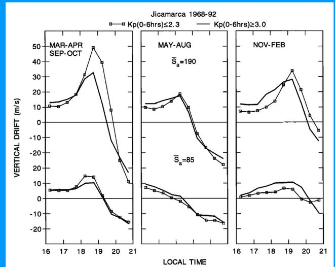
Figure 2. Variation of the vertical drift velocity for periods of low (bottom panels) and high solar flux (upper panels) in geomagnetic quiet (lines with squares) and perturbed conditions (continuous lines) for different seasons[[1]]. Note that for the June solstice (center panel), the vertical velocity does not reach values that could produce the ionosphere instability that causes the spread-F phenomenon. Figure adapted from[1].
